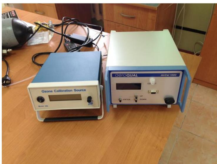
Figure 2 Left: 306 ozone calibrator from 2B Tech instruments, Right: Aeroqual Aircal 1000
