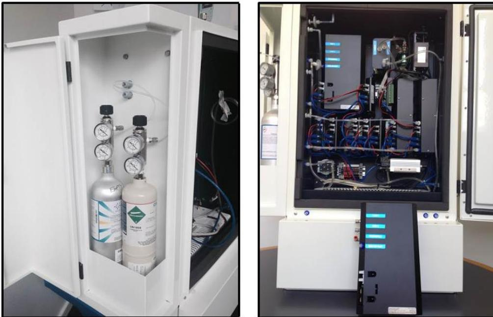
Figure 1 The integrated AirCal 8000 for automated gas delivery
